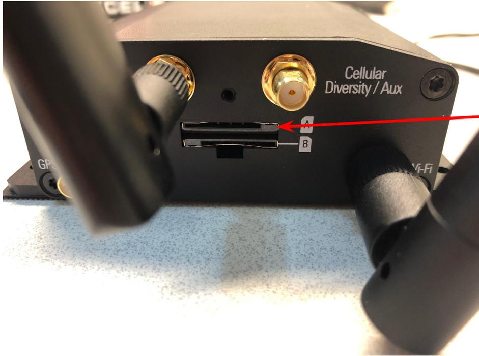
The slot for the SIM card is located on the side of the modem where the antennas connect.
